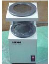
the "STRESS EQUIPMENT". To solve the stress points, please mark with Text pens on major "Stress" point on lens pattern. Then polish the pattern a little bit till the stress point as less as possible. As per to avoid the "Rainbow", please reduce the lens size as small as possible.
